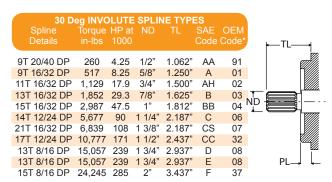
HP at 1000 RPM. Torque and HP requirements noted are typical (based on shaft St of 25000 PSI) and should be considered as a guide only. Torsional stress is calculated at spline undercut.
