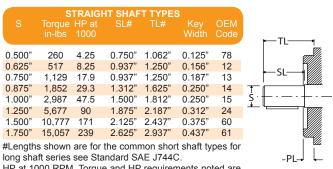
HP at 1000 RPM. Torque and HP requirements noted are typical (based on shaft St of 25000 PSI) and should be considered as a guide only.
