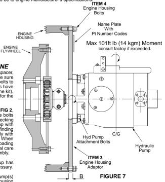
**STEP 5.** After positioning the driveplate Item 1 into the flywheel, select the flywheel bolts supplied in Item 4 and make sure they are the correct size, thread and length to suit the application. We recommend that Loctite 242 or 243 should be used to secure the bolts additional to the star shake proof washers provided in item 4. Bolt torque values should be to engine manufacturer's specifications.
