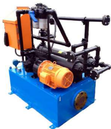
Oil cooling package fitted with shell and tube heat exchangers, oil tank, Haight pump, duplex filter, 3 way thermostatic control. Sensors for oil flow, oil level, oil temperature, oil pressure, oil moisture content and filter condition.
