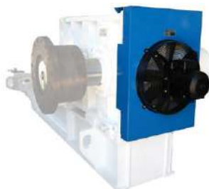
Versacool model Air Delivery Group fitted to a custom enclosure for air cooling the exterior of a conveyor gearbox.
